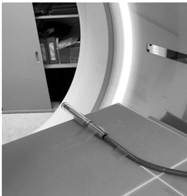
Figure 2. Experimental setup of the absolute dose measurement. The chamber with the build-up cap is located at the isocentre, and the amount of charge is measured
